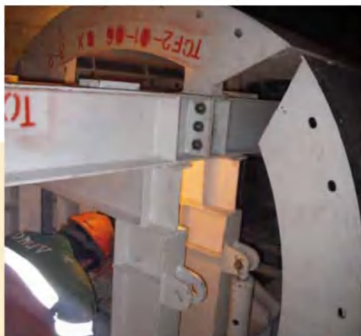
Project: HongKong drainage Tunnel User: Shanghai DCW Trading Company Limited Technical Data: length 9m; radii 1.25m; weight of trolley 17t workshop photograph
